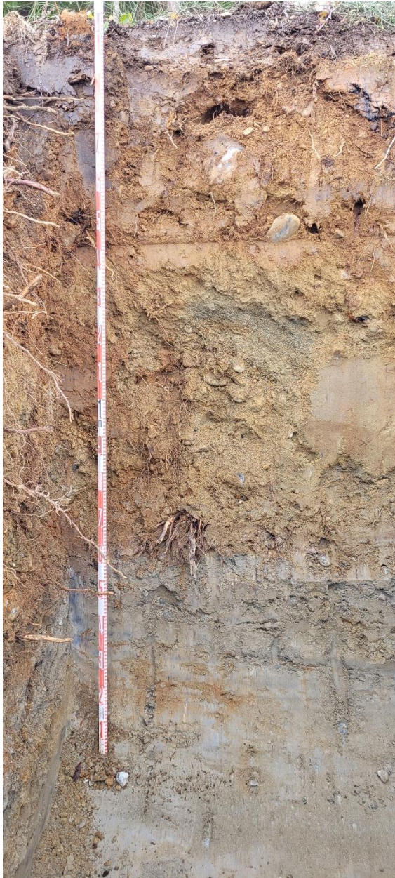
PHOTO 2. PROFILE OF TEST PIT 2 EXCAVATED TO INFORM THE AQUIFER PROTECTION PLAN DEVELOPED BY MADRONE ENVIRONMENTAL SERVICES. PHOTO DATED FEBRUARY 22, 2023.
