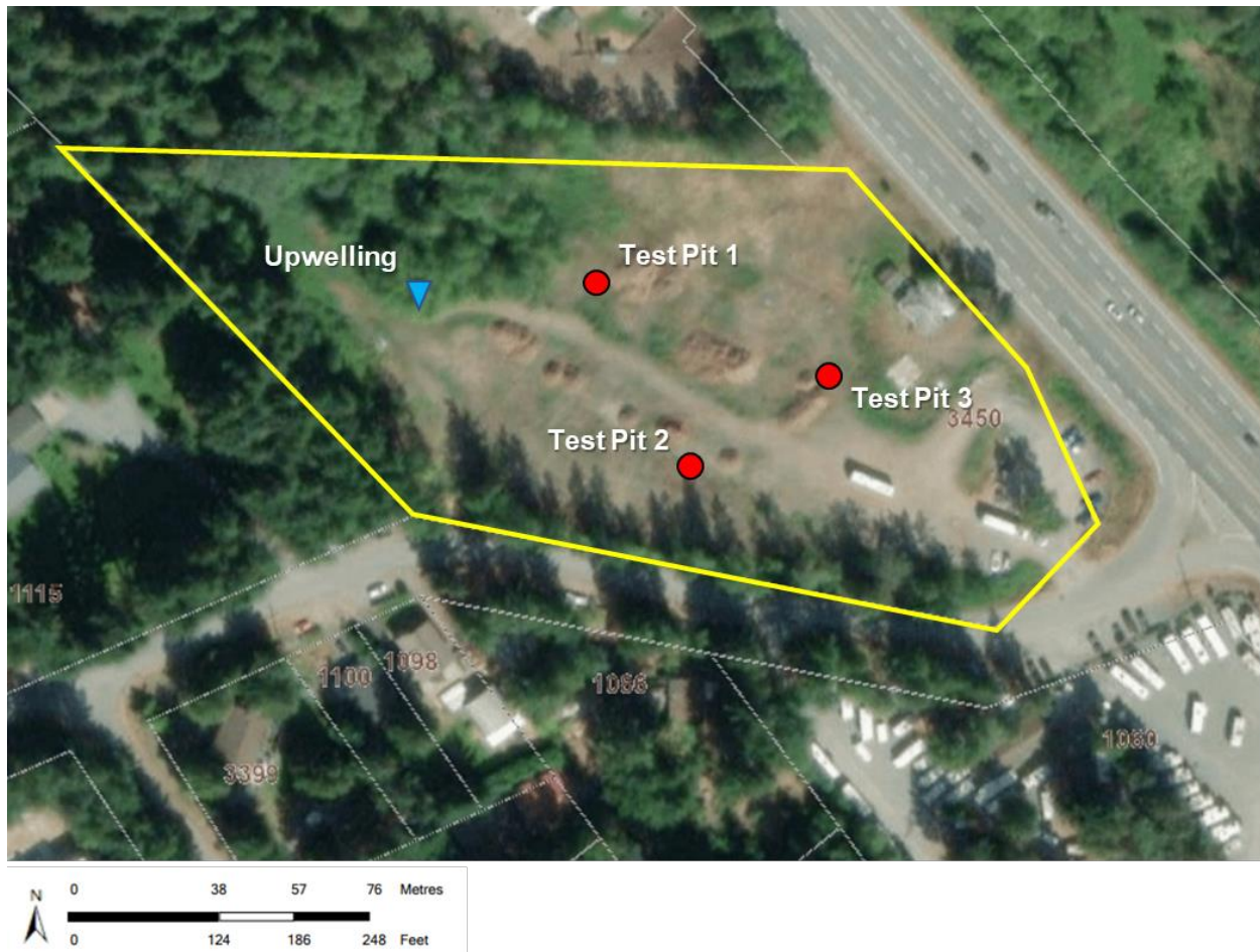
FIGURE 1. AERIAL VIEW OF 3450 TRANS CANADA HIGHWAY (OUTLINED IN YELLOW). THE LOCATIONS OF THE TEST PITS EXCAVATED FOR MADRONE ENVIRONMENTAL SERVICES' ASSESSMENT TO INFORM AN AQUIFER PROTECTION PLAN AS RED PLACEMARKS. THE LOCATION OF GROUNDWATER UPWELLING INTO A SMALL POOND OBSERVED BY MADRONE IS MARKED. IMAGERY PROVIDED BY THE COWICHAN VALLEY REGIONAL DISTRICT (WORLD VIEW).
